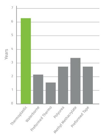
\*GDOT 2015, Striping on Asphalt, 10,000 ADT, Service Life to 250 mcd/m2/lux
